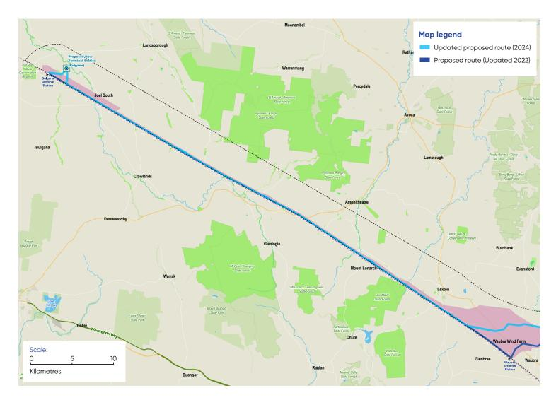
The proposed route from Bulgana to Waubra travels east from the existing Bulgana Terminal Station to the site of a new 500kV terminal station before heading south to join the existing transmission line easement. The route then runs parallel to the existing Ballarat to Horsham transmission line.
